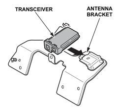
18. Using the 6 mm screws, secure the bidirectional antenna to the antenna bracket.
