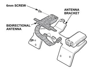
19. Plug the bidirectional antenna into the transceiver and secure the clip on the harness to the bracket.
