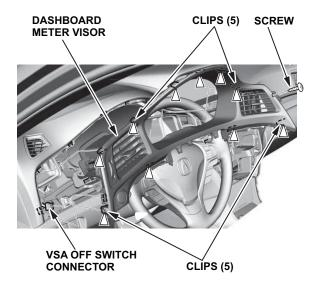
14. Remove the gauge control module and disconnect the gauge control module connector.
