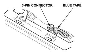
17. Slide the transceiver onto the antenna bracket as shown.
