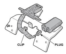
20. Using the two flange nut's attach the antenna bracket assembly to the dashboard support.
